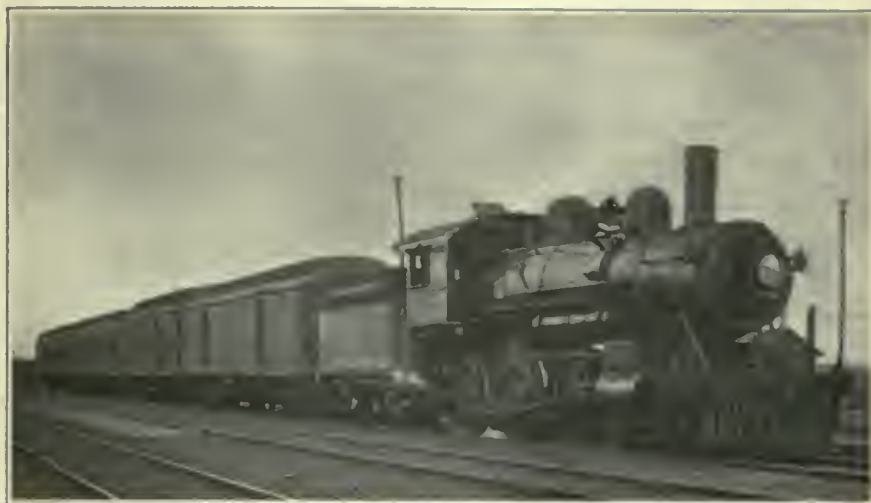
FIG. 370. SUBURBAN PASSENGER TRAINS. Suburban Train of the Chicago & North Western Railway at Proviso. This train consists of a ten-wheel locomotive and four coaches.
